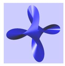
Fig. 1. Example of a tangent developable
